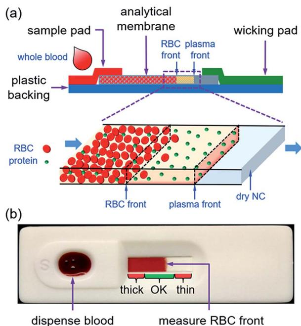
Fig. 1 No-reaction lateral flow assay (nrLFA) schematic.
