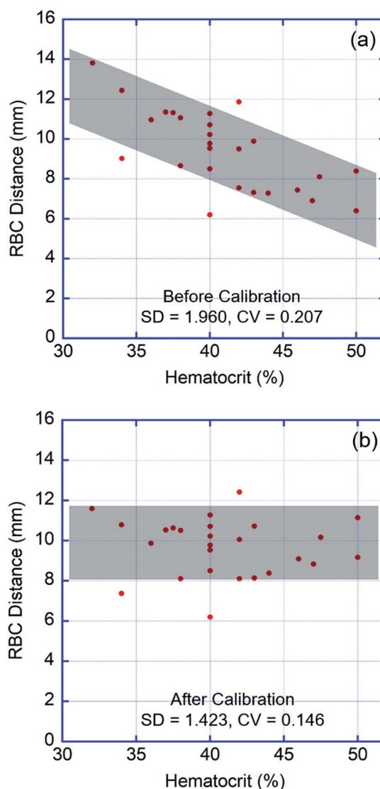
Fig. 3 Data scatter of RBC distance vs. Hct for all patients: (a) before calibration; (b) after calibration ( $t = 4$  min).
