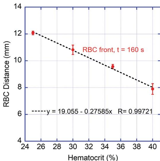
Fig. 2 RBC distance vs. hematocrit when using 30  $\mu\text{L}$  of citrated rabbit blood with 25%, 30%, 35% and 40% Hct (mean  $\pm$  SD,  $n = 10$ ).<sup>24</sup>
