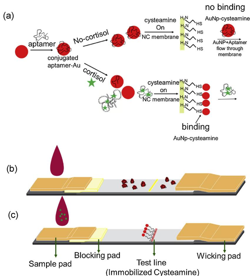
Fig. 8. Cortisol detection on lateral flow assay using AuNP-aptamers: (a) basic concept; (b) illustration of negative control - no color change in absence of cortisol; (c) color change in test line in presence of cortisol.
