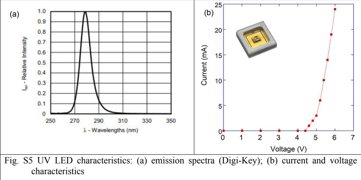
Fig. S5 UV LED characteristics: (a) emission spectra (Digi-Key); (b) current and voltage characteristics
