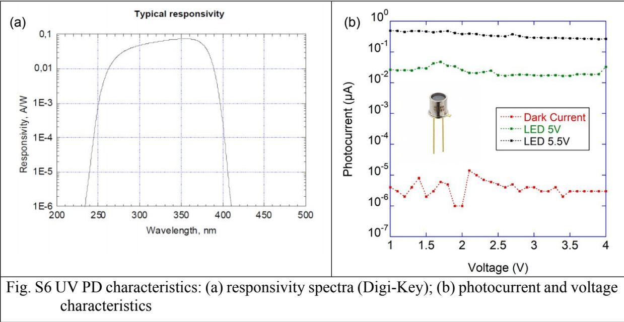
Fig. S6 UV PD characteristics: (a) responsivity spectra (Digi-Key); (b) photocurrent and voltage characteristics
