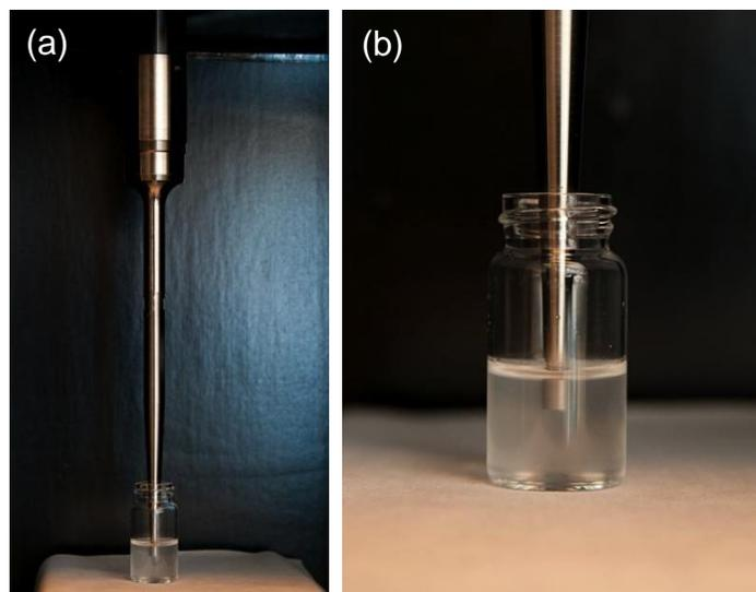
Figure 3. Sonication process used to reduce the DNA molecular weight: (a) Misonix S-4000 sonicator; (b) close-up of sonic horn tip.
