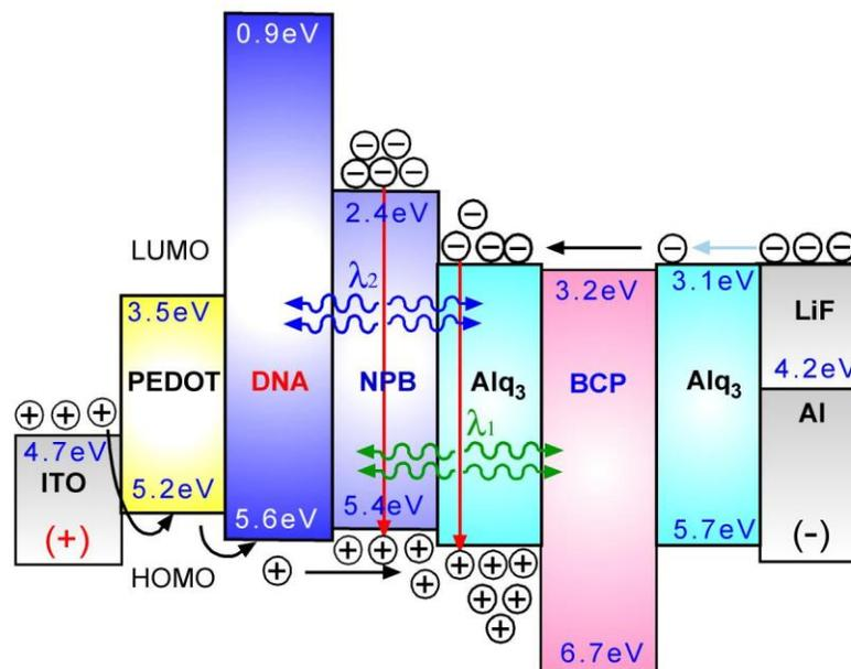
Figure 7. The completed DNA OLED in operation (top) and HOMO-LUMO levels showing the electron blocking properties of the DNA layer [4].
