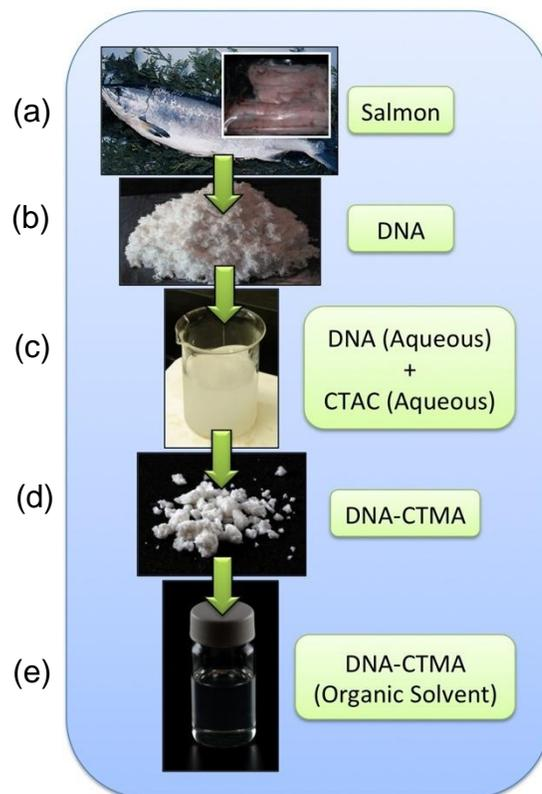
Figure 2. Natural purified DNA is extracted from salmon, purified, freeze-dried, and sonicated. The surfactant CTAC is added to produce the DNA-CTMA complex which not soluble in water but is soluble in organic solvent. At this point the DNA is ready for thin film fabrication [2].
