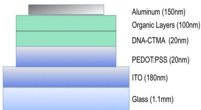
Figure 1. Schematic diagram of typical BiOLED structure, including layer thicknesses.
