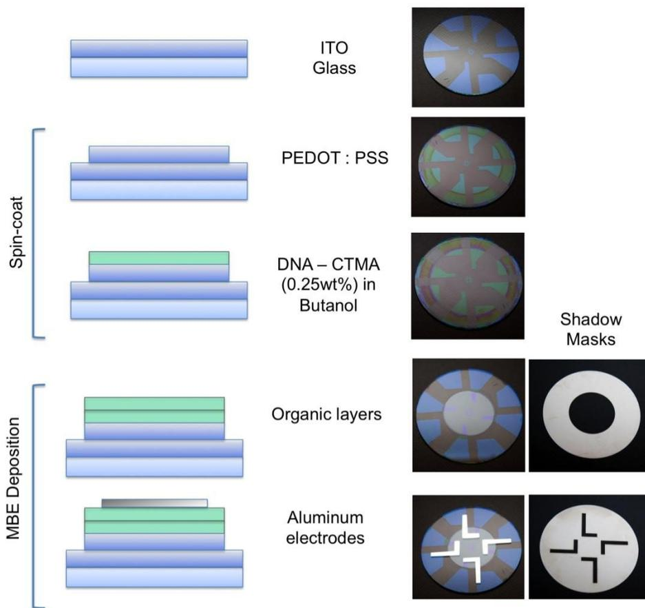
Figure 5. The process of the fabrication of OLED includes the first section of spin-coating PEDOT:PSS and DNA-CTMA; the final steps deposit the remaining organic layers and the aluminum electrodes via thermal evaporation.
