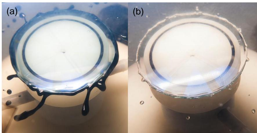
Figure 4. Spin-coating process of layers in BiOLED structure: (a) PEDOT:PSS; (b) DNA-CTMA.
