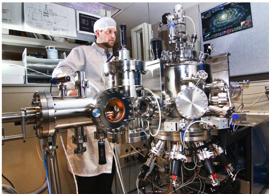
Figure 6. MBE vacuum deposition system to deposit highly purified organic layers and electrodes. The load lock is located on the left half of the system and the main chamber is on the right. The main chamber contains 7 effusion cells located on the bottom flange of the chamber.
