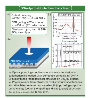
grating etched into the  ${\rm SiO}_2$  layer over which a DNA - (cationic) surfactant-dye layer was deposited. The dye we chose was sulforhodamine (SRh), an anionic dye used extensively in dye lasers with strong red emission. The DFB grating had a period of 437 nm, which corresponded to the  $2^{\rm nd}$  order emission at the SRh amplified spontaneous emission wavelength of 650 nm.
