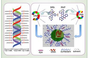
(Left) Natural DNA-Na salt in aqueous solution is transformed into DNA-surfactant salt, which is insoluble in water but soluble in organic solvents. (Right) Dye molecules interacting with DNA-surfactant complex.
