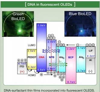
(Top) Green- and blue-emitting BiOLEDs (bottom) HOMO/LUMO energy levels in OLED structure showing the electron blocking function of the DNA layer; electroluminescence occurs in either the AIQ<sub>3</sub> (green) or NPB layer (blue) layers. Source: J. A. Hagen et al. Appl. Phys. Lett. **88**, 171109 (2006).
