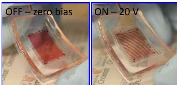
Figure 7. EW array on a flexible plastic substrate.
