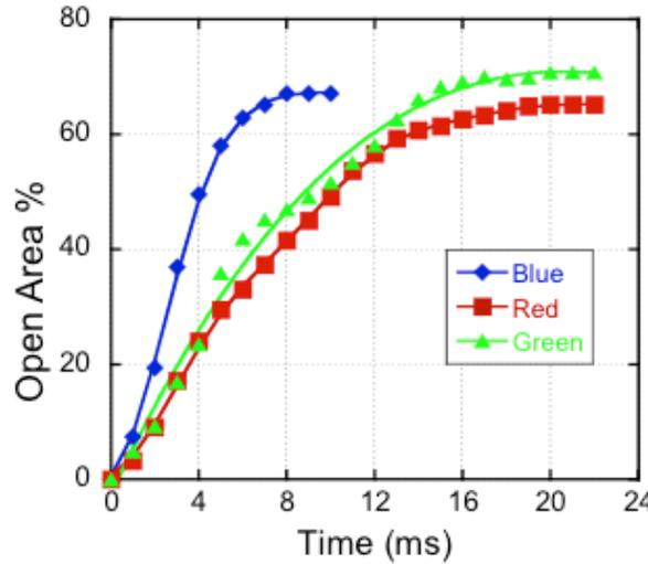
Figure 5. Open area as a function of time for each level in a multi-color vertical stack array<sup>11</sup>.
