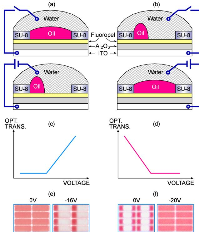
Figure 1. Operation of EW devices<sup>9</sup> with normal process (left column) and with plasma/anneal process (pEW – right column): (a, b) device schematics under floating (or zero) and negative voltage; (c, d) trend in optical transmission with applied voltage; (e, f) photographs of EW arrays under zero and negative voltage.
