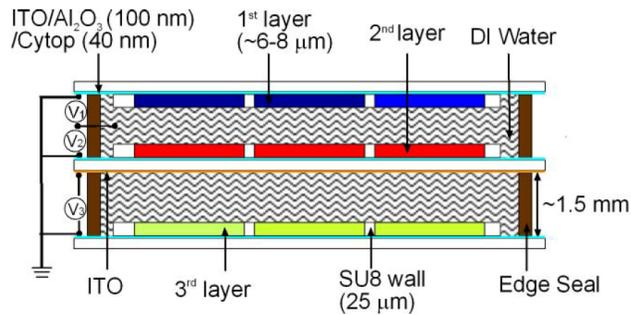
Figure 3. Three-color EW array using the vertical stack approach<sup>11</sup>.
