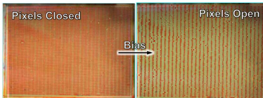
Figure 4. Switching of EW array with  $45 \times 21$  pixels under applied bias.
