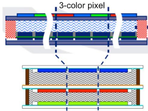
Figure 2. Implementation of three-color EW displays using the side-by-side filter approach (top) and the multi-layer vertical stack approach (bottom).
