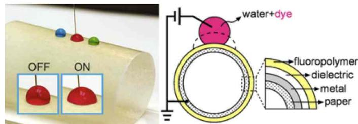
Figure 6. EW on a rolled paper substrate<sup>12</sup>.
