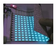
ON DISPLAY: Paper can be used to make displays that either reflect incoming light or emit their own. One way to make a reflective display is to alter the surface tension of liquid pixels [top]. Organic light-emitting diodes can also be built on paper to make displays that glow [bottom].
