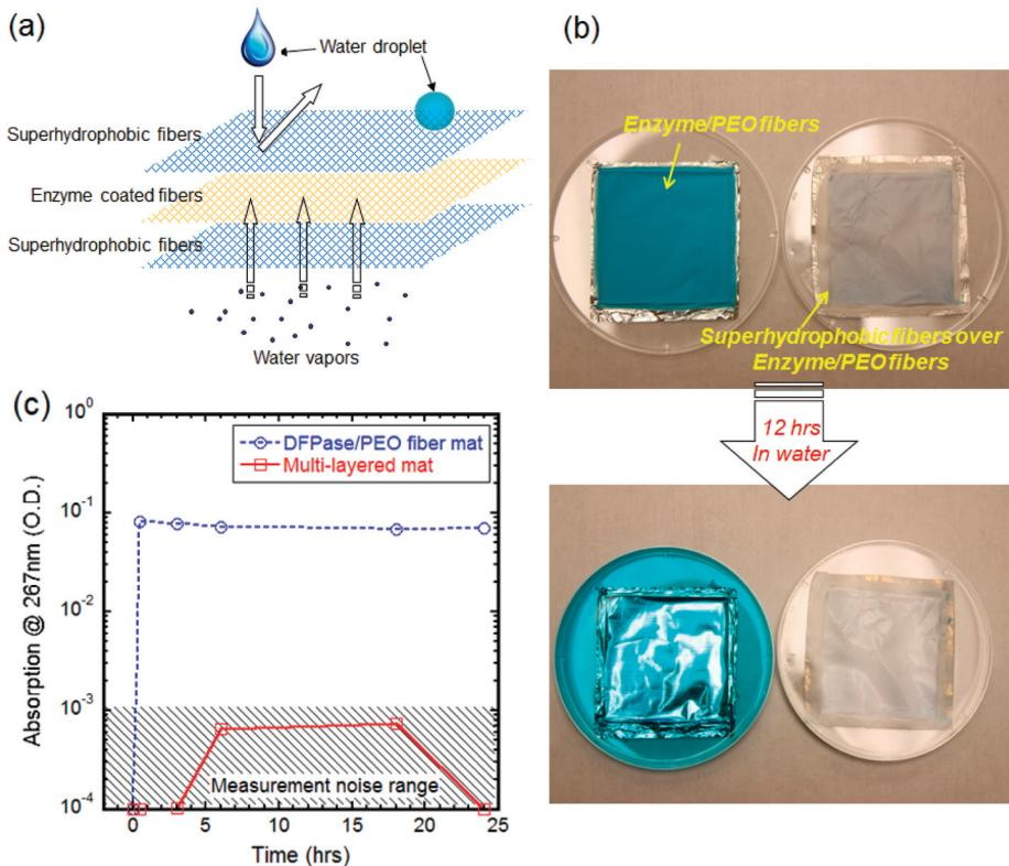
**Figure 9.** Multilayer fiber mat with outer superhydrophobic fibers and inner enzyme containing fibers: (a) schematic of multilayer fiber mat; (b) demonstration of multilayer protection of enzyme containing fibers; (c) absorption (at peak wavelength  $\sim 267$  nm) vs time, comparison between enzyme/PEO fiber mat and multilayer fiber mat.
