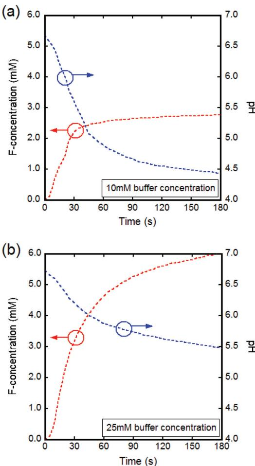
**Figure 6.** Dependence of DFP-DFPase reactions on pH change in solution: 2.5 mg of DFPase added in 10 mL of PIPES buffered DFP solution made of 3 mL of 25 mM DFP solution and 7 mL of (a) 10 or (b) 25 mM PIPES buffer solution. Measurement repeated 3 times and averaged graphs are shown.
