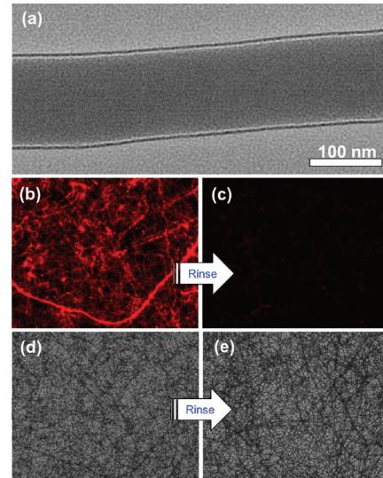
**Figure 2.** (a) Core–sheath structure observation using TEM; and fluorescence microscopy of coaxial fibers containing Keystone Red dye in the sheath, before and after rinsing with water: (b) initial dark-field image, (c) dark-field image postwashing, (d) initial bright-field image, (e) bright-field image postwashing. Exposure times for bright-field and dark-field modes are 2 ms and 2 s, respectively.
