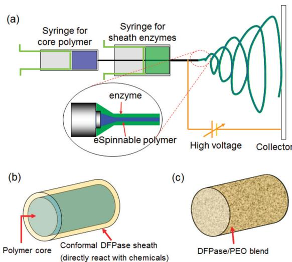
**Figure 1.** Electrospinning of enzyme containing fibers: (a) coaxial dual solution electrospinning; (b) core–sheath coaxial fiber with polymer core and conformal DFPase containing sheath; (c) uniform DFPase/PEO blended fiber using single solution electrospinning.
