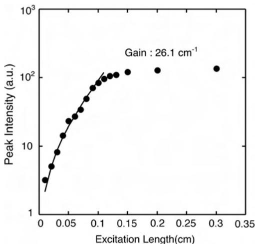
**Figure 6** Optical gain obtained from Eu doped GaN layer grown on *glass* substrate. Peak wavelength of emission is ~620 nm. The sample was pumped by N<sub>2</sub> laser with 3.73 MW/cm<sup>2</sup> at 337 nm.
