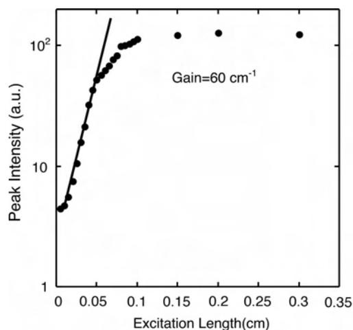
**Figure 4** Optical gain obtained from Eu-doped GaN layer with AlN top and bottom cladding layers grown on *silicon* substrate. Peak wavelength of emission is  $\sim 620 \text{ nm}$ . The sample was pumped by N<sub>2</sub> laser with 3.73 MW/cm<sup>2</sup> at 337 nm.
