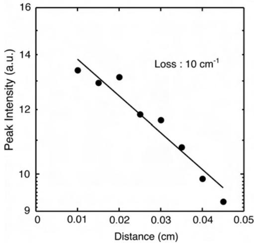
**Figure 5** Optical loss obtained from Eu doped GaN layer with AlN top and bottom cladding layers grown on *silicon* substrate. Peak wavelength of emission is ~620 nm. The sample was pumped by N<sub>2</sub> laser with 3.73 MW/cm<sup>2</sup> at 337 nm.
