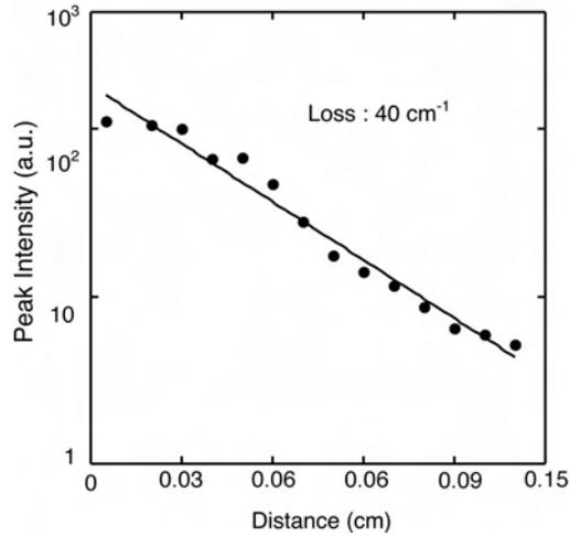
**Figure 7** Optical loss obtained from Eu doped GaN layer grown on glass substrate. Peak wavelength of emission is ~620 nm. The sample was pumped by N<sub>2</sub> laser with 3.73 MW/cm<sup>2</sup> at 337 nm.
