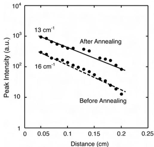
**Figure 3** Peak stimulated intensity signal as a function of distance (using the SES technique [4]) for determining the loss in GaN:Eu cavities grown on *sapphire* with and without post-growth anneal. The Eu cell temperature was 470 °C corresponding to Eu concentration of  $\sim 1 \text{ at}\%$ .
