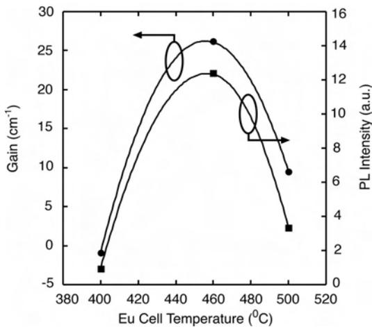
**Figure 1** Effect of Eu cell temperature (and consequent concentration) in the GaN layers grown on *sapphire* on photoluminescence (PL) intensity (using CW He–Cd laser at 325 nm) and on gain obtained with the variable stripe length (VSL) technique (using pulsed N<sub>2</sub> laser at 337 nm).
