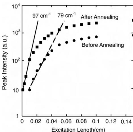
**Figure 2** Peak stimulated intensity signal as a function of excitation length (using the VSL technique) for determining the gain in GaN:Eu cavities grown on *sapphire*, with and without post-growth anneal. The Eu cell temperature was 470 °C corresponding to Eu concentration of  $\sim 1 \text{ at}\%$ .
