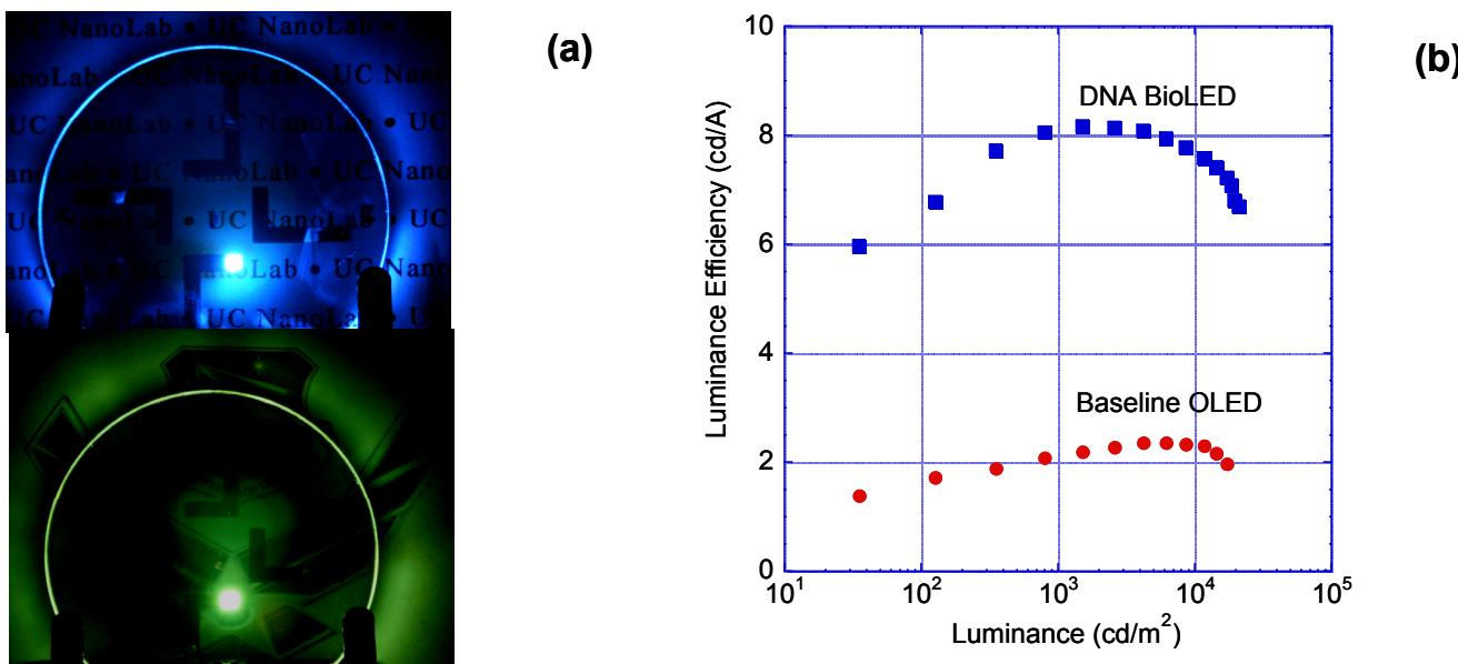
**Figure 4.** DNA BioLEDs: (a) blue (NPB) and green ( $\text{Alq}_3$ ) emitting devices in operation; (b) luminance efficiency versus luminance for green emitting BioLED and for conventional baseline OLED.
