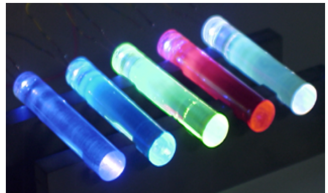
Fig. 15. Photographs of (left to right) violet, blue, green red, and white Hybrid I/O lamps. The violet lamp has no lumophore and appears in false color (photographed with 3-color CCD). (Color version available online at http://ieeexplore.ieee.org .)
