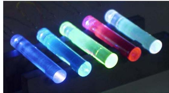
Figure 2. Photograph of violet (no CCM), blue, green, red, and white hybrid I/O lamps.
