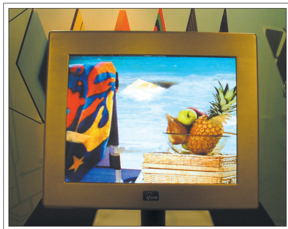
Fig. 2: iFire Technology's current 17-in. TDEL prototype exhibits higher luminance, resistance to differential aging, and greater manufacturing simplicity, thanks to the company's Color-by-Blue approach.
