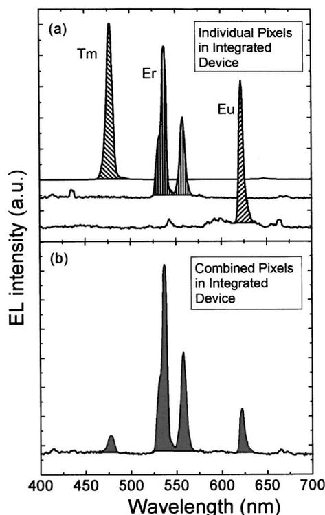
FIG. 4. EL emission spectra from integrated blue, green, and red pixels of GaN:RE: (a) individual spectra from Tm, Er, and Eu pixels at a dc bias of 30 V with current of 33, 3, and 5 mA, respectively; (b) spectrum from all three pixels with simultaneous emission, at a dc bias of 30 V and current of 45 mA.
