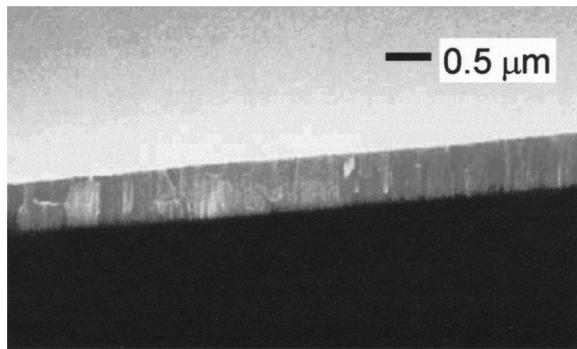
FIG. 1. Cross-sectional SEM micrograph of  $\sim 0.6 \mu\text{m}$  SOG layer on Si wafer.
