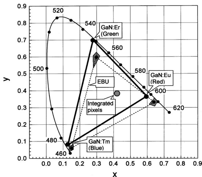
FIG. 5. CIE  $x$ - $y$  chromaticity diagram showing the locations of the blue, green, and red emission from the individually biased pixels in an integrated device and from simultaneously biasing all three pixels in the device. Also shown are the coordinates of the EBU-recommended phosphors.
