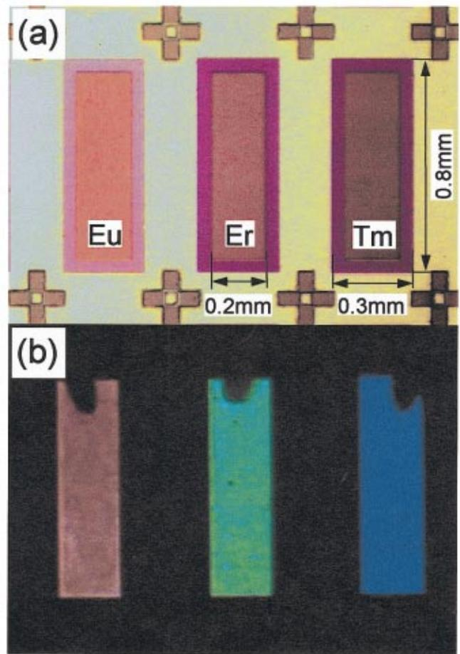
FIG. 3. (Color) Laterally integrated GaN:RE TFEL containing the three primary colors fabricated with the SOG lift-off technique: (a) optical microscopy photograph of the GaN TFEL showing the three-color integration; (b) blue, green, and red emission under dc bias from TFEL GaN devices doped with Tm, Er, and Eu, respectively.
