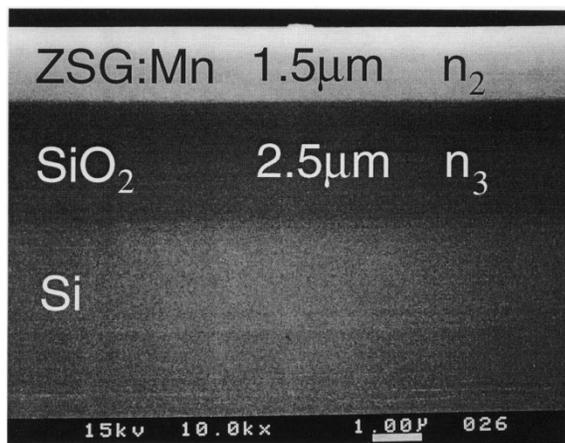
Fig. 1. SEM photomicrograph showing the cross section of a ZSG:Mn planar waveguiding structure.
