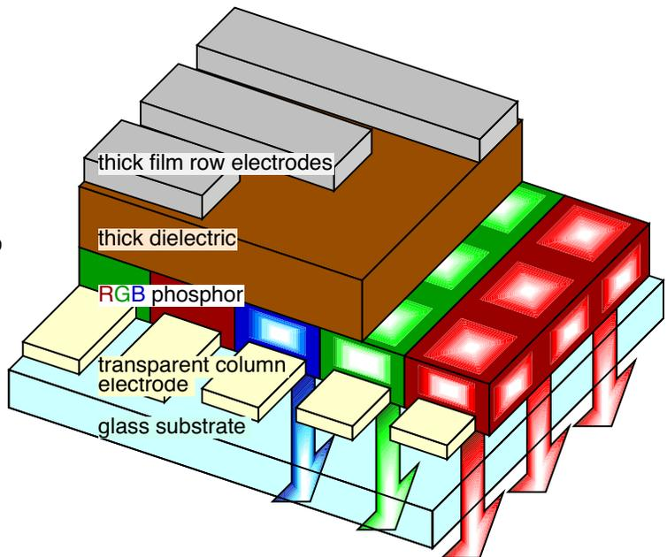
Fig. 8 Schematic of full-color TDEL display structure.
