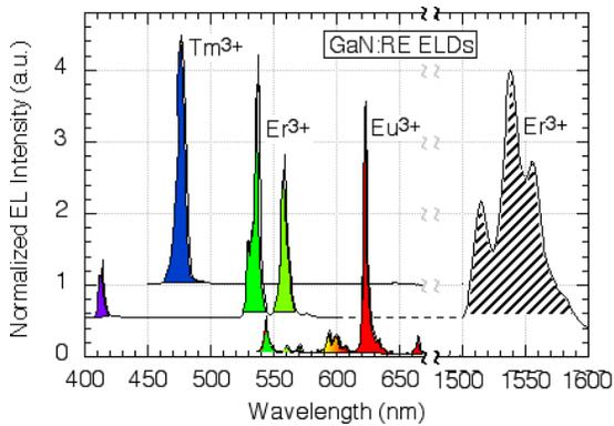
Fig. 3 The emission spectra of Tm-, Er-, and Eu-doped GaN ELDs showing the visible and IR wavelengths of interest.
