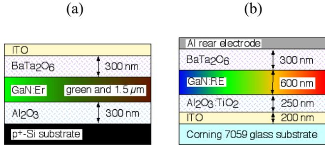
Fig. 5 Schematic diagrams of example AC-ELDs formed on Si substrates (a) and glass substrates (b). The device in (a) can also be utilized as a 1.5 μm emitter on Si.
