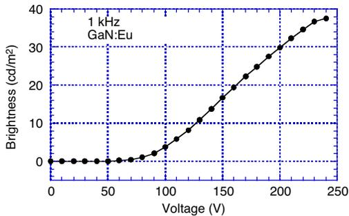
Fig. 7 Brightness characteristics of GaN:Eu TDEL as a function of voltage.
