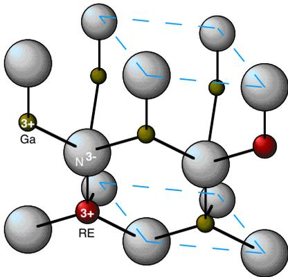
Fig. 1 Simple model of GaN:RE crystal structure.
