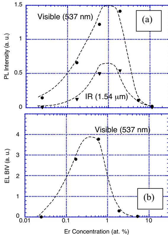
Fig. 2 PL and EL intensity vs. Er concentration: (a) visible and IR PL intensity; (b) current normalized visible EL (BIV).
