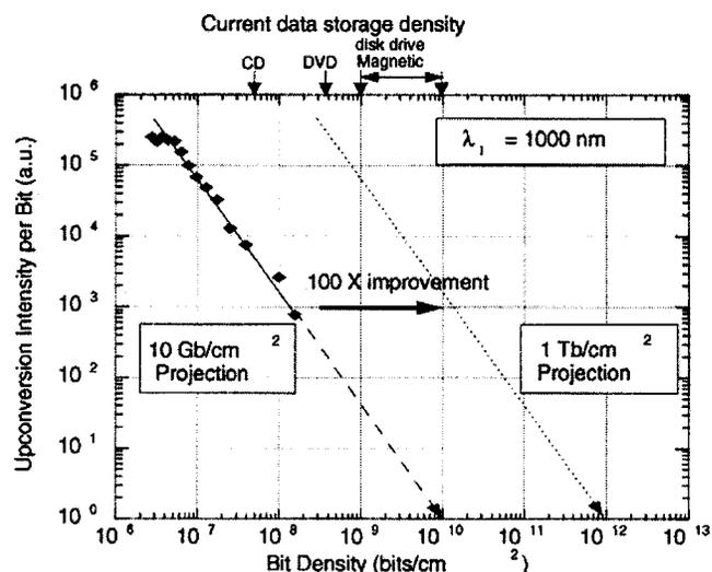
Fig. 4 Upconversion emission intensity versus current bit density (diamond data points). Maximum bit density of  $\sim 10\text{ Gbits/cm}^2$  is projected with current FIB milling parameters. To achieve terabyte storage capacity, a  $100\text{X}$  improvement is required.
