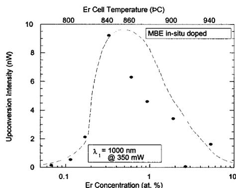
Fig. 3 Upconversion emission intensity of Er-doped GaN as a function of Er cell temperature and corresponding concentration.
