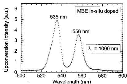
**Fig. 2** High-resolution spectrum of green upconversion luminescence in an in-situ Er-doped GaN film excited by a laser at 1000 nm.
