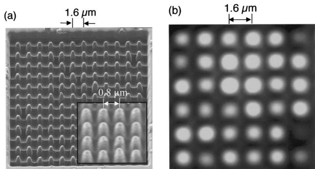
**Fig. 1** 1(a) Microphotographs of 1.6- $\mu\text{m}$ -pitch and 0.8- $\mu\text{m}$ -pitch bit patterns. (b) CCD optical image of upconversion emission from 1.6- $\mu\text{m}$ -pitch bit pattern.
