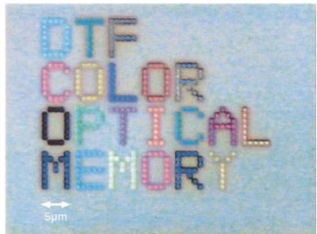
FIG. 4. (Color) Color reflected light photograph of a fabricated DTF memory structure taken using a 100\times objective lens and a CCD camera. The 16 depth levels produced 16 distinct colors.
