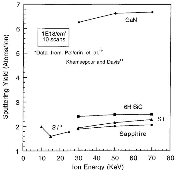
FIG. 4. Comparison of the sputtering yield of GaN, Al<sub>2</sub>O<sub>3</sub>, SiC, and Si (dose: 1 × 10<sup>18</sup> cm<sup>-2</sup>, normal incidence, 10 scans).
