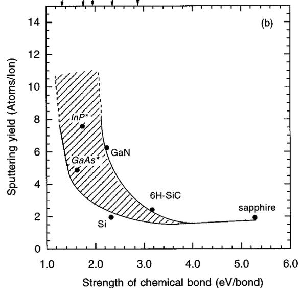
FIG. 5. Milling rate and sputtering yield of selected materials as a function of bond strength. The experimental data are for 30 keV Ga<sup>+</sup>, 10 scans from this work (GaN, SiC, Si, Al<sub>2</sub>O<sub>3</sub>) and from Young *et al.* (Ref. 14) (GaAs and InP). Also shown are the bond strengths of other semiconductors of interest.
