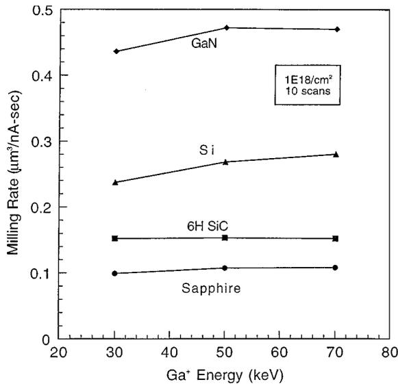
FIG. 3. Comparison of Ga<sup>+</sup> milling rate of GaN and that of potential substrate materials (Al<sub>2</sub>O<sub>3</sub>, SiC, Si) as a function of ion energy (dose: 1 × 10<sup>18</sup> cm<sup>-2</sup>, normal incidence, 10 scans).
