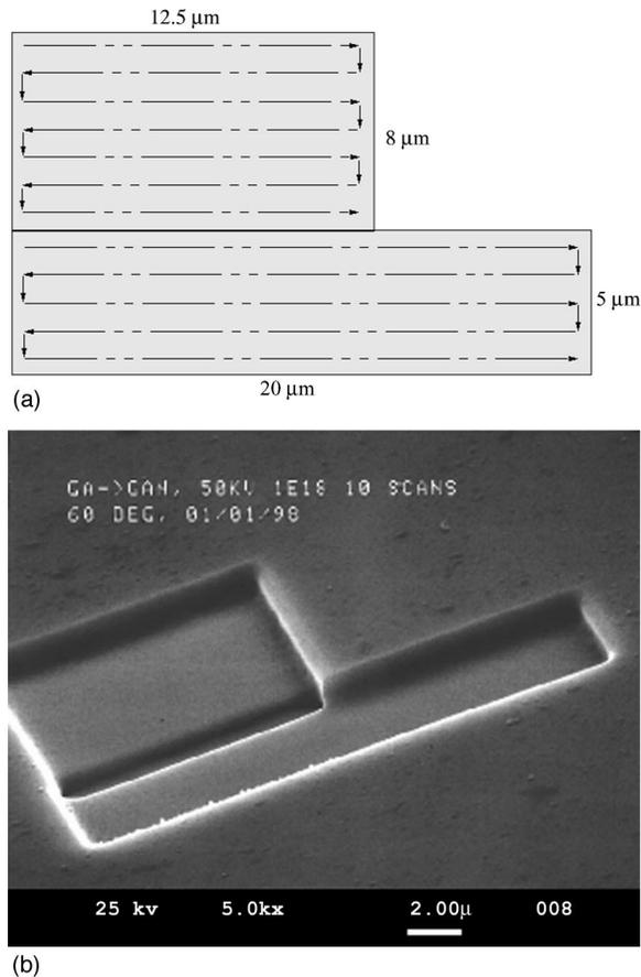
FIG. 1.  $\text{Ga}^+$  FIB micromilled pattern: (a) schematic of the pattern and the serpentine scan; (b) SEM photograph of the GaN pattern micromilled using a 50 keV  $\text{Ga}^+$  FIB with a dose of  $1 \times 10^{18} \text{ cm}^{-2}$ , at normal incidence, over 10 scans.
