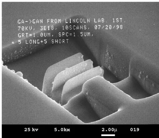
Fig. 6. SEM photograph of the GaN short cavity laser with DBR gratings fabricated by FIB micromilling: 70 keV  $\text{Ga}^+$ ,  $3 \times 10^{18} \text{ cm}^{-2}$  dose, normal incidence. The center-to-center spacing of the individual mirrors is  $2.5 \mu\text{m}$ .
