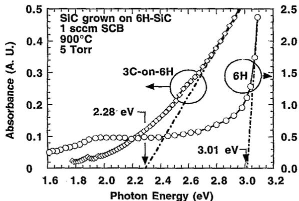
FIG. 1. Optical absorption spectra of 6H-SiC substrate and of sample with film grown at 900 °C with SCB on a 6H-SiC substrate.
