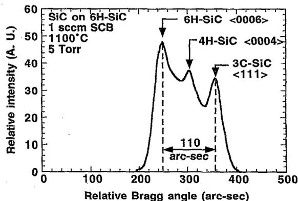
FIG. 3. DCXRD spectrum of sample with 3C-SiC film grown with SCB at 1100 °C on 6H-SiC substrate.
