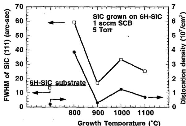
FIG. 2. Effect on film growth temperature on the full width at half maximum (FWHM) signal of SiC (111) double crystal x-ray diffraction (DCXRD) peak and on the corresponding dislocation density. Values for as-received 6H-SiC substrate also shown.
